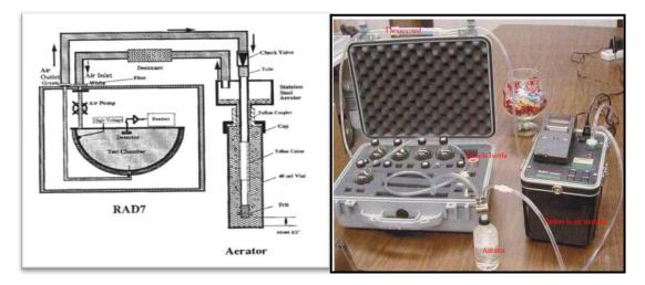
Fig. 3: Schematic diagram of RAD7, a solid state, ion implanted, planar Silicon alpha detector with RAD H2O assembly in (Durridge Company Inc., 2012)
